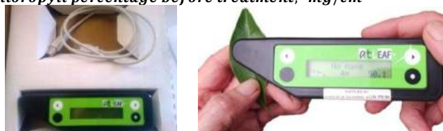
Fig.27: Digital Chlorophyll Meter model atLEAF.
