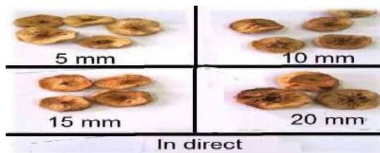
Fig.16 Apple slices color change by drying in indirect system for different thicknesses.
