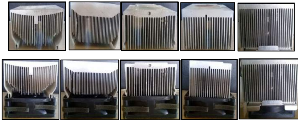
Fig (1): types of heat think with and without fan. Local Heat sink to cooling the LEDs.
