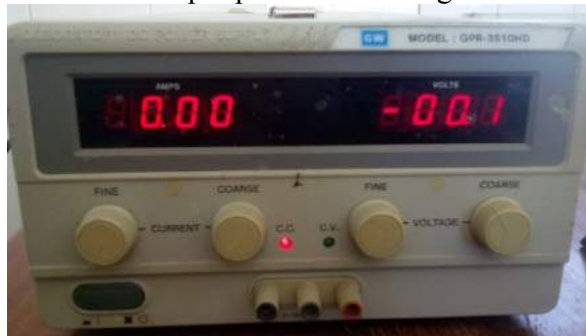
Fig (4): DC power supply (GPR-3510HD).
