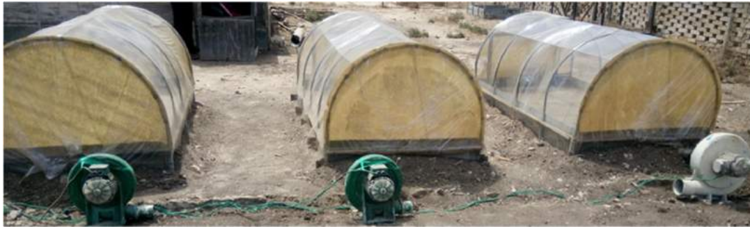
Plate (1): The three identical solar dryers used for the experimental work.
